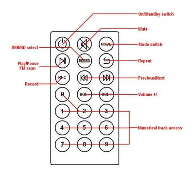
In addition to the panel controls, an infra-red remote control is provided for the USB/SD player which adds some further functions to allow greater control over the media player.
